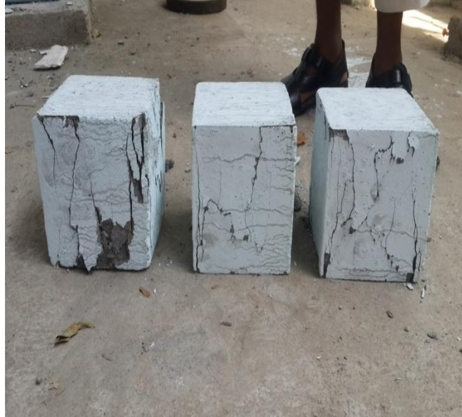
Figure 2. Cubes after testing
